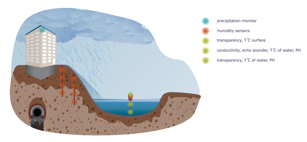
Another aspect of Project "Atmosphere" is connected to hydrological measuring devices in order to monitor the water cycle in nature and to study its purity. Consider a building built on a slope. Under the building are installed drains and in the soil are humidity sensors. These sensors are required to record the stability and density of land that is washed away by groundwater and rainwater. If the soil is "soft" - the risk of collapse, landslide or destruction of buildings increases.
